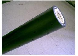
Introduced after testing on numerous horizontal well installation projects, EnviroFlex was designed specifically for direct-pull (as opposed to carrier casing) horizontal well installations. Using a composite filtration system, comprising a non-woven geotextile, a geogrid supporting mesh or a porous polyethylene tube bonded to the *inside* of a perforated well screen, and an inner PVC screen, EnviroFlex maintains high tensile strength
