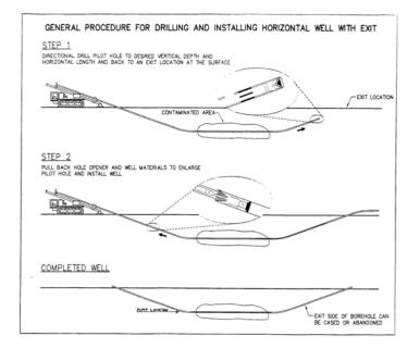
The drillhead is directed downward along a pre-planned path so that at the desired location the well screen portion of the borehole is flat or inclined at a specified grade. The borehole is advanced along the well screen portion and then back to the surface.
