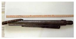
head. The duckbill or cutting bit attaches to the front of the drill head at a tapered angle. It is this angle that causes the drill head to change direction of travel when thrusting forward with no rotation.
