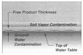
The solution to this is to design a dual-phase extraction system that can withdraw either free product or a mixture of free product and water (which is run through an oil-water separator prior to treatment) when the water table is high, or soil vapor when the water table drops. Dual-phase extraction systems are gaining popularity with designers, particularly as more advanced pumps, separators and treatment systems are being developed.
