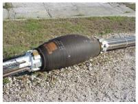
One method to ensure the well annulus is blocked is to install a pneumatic packer in line with the well materials. The advantage of a pneumatic packer is that it can be installed a long way from the well ends and it completely blocks the annulus. The primary disadvantage is the air lines needed to inflate the packers. The air lines are relatively weak and often do not survive the pullback.
