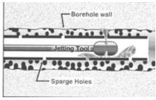
Engineers should consider the use of well screens with an integral filter to avoid this problem, or they can place the properly designed air sparge pipe inside a larger-diameter, conventional well screen. In the first case, development becomes less critical because fine-grained soil is prevented from entering the well. The carrier casing method also has merit because the well can be properly developed; then the sparge pipe can be inserted afterwards.
