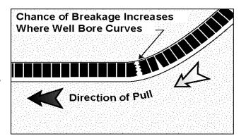
usually as the casing flexes through a curve in the well bore path, as shown at right. Stress transmitted along the stiff pipe is focused at this joint, causing breakage or buckling of the rods at the weld.
