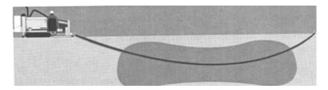
Once it exits the ground, the drill head is removed and a back reamer or expander is attached along with a swivel and the slotted well screen. It is then pulled back through the pilot bore to the drilling unit. To better understand it, let's take a look at the individual pieces of the process.
