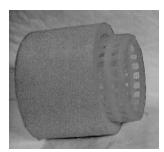
A filter screen constructed of sintered polyethylene resin beads, Schumasol was developed to maximize the open area of the screen while maintaining filtration properties that meet or exceed pre-pack performance. It achieves excellent filtration characteristics, but the porous construction of the screen limits its tensile strength. Installation using a carrier casing is specified by the manufacturer. Schumasol has been successfully installed on several major remediation projects in the U.S.
