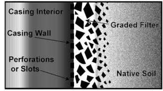
to the well screen, creating a graded filter, from coarse to fine, that extends outward from the screen to the well bore.
