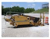
rotation, forward thrust, and pullback. The industry-wide standard for rating the size of a machine is the total pounds of pullback capability. Directional drilling machines typically used for environmental applications are categorized as small
