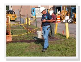
feet, depending on site conditions. We have walkover and remote systems available, and can typically maintain an accuracy of approximately two inches down to a depth of approximately 12 feet. Below 12 feet, we often maintain an accuracy of two percent.
